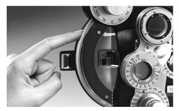
Figure TM-3 Moving Weak Sphere Dial
