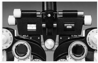
Figure TM-1 Vergence Levers Out (Distance Tests)
