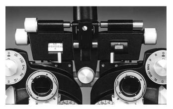
Figure TM-2 Vergence Levers In (Near Tests)
