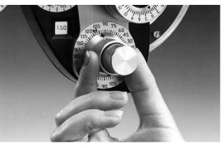
Figure TM-6 Turning Cylinder Axis Knob
