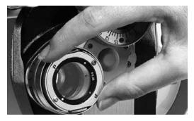
Figure JC-6 Rotate Cross Cylinder
